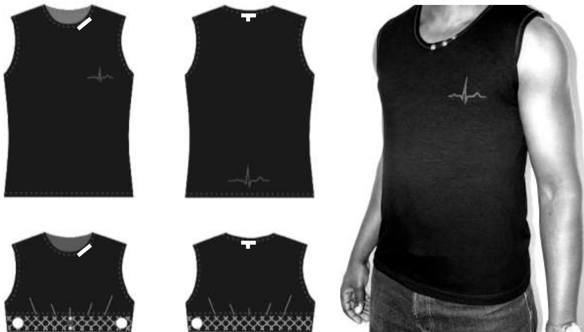
Fig. 4. Sensory shirt with inner and outer part (left panel); proband wearing a prototype of the sensory shirt where the functionality is only visualized by the ECG symbol (left and right panel).
