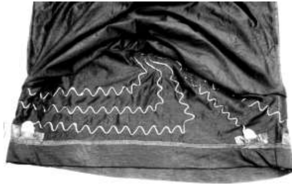
Fig. 5. Inner shirt with stainless steel filament yarns sewn on the shirt in an undulating form, contacting the ECG electrodes and the other sensors.
